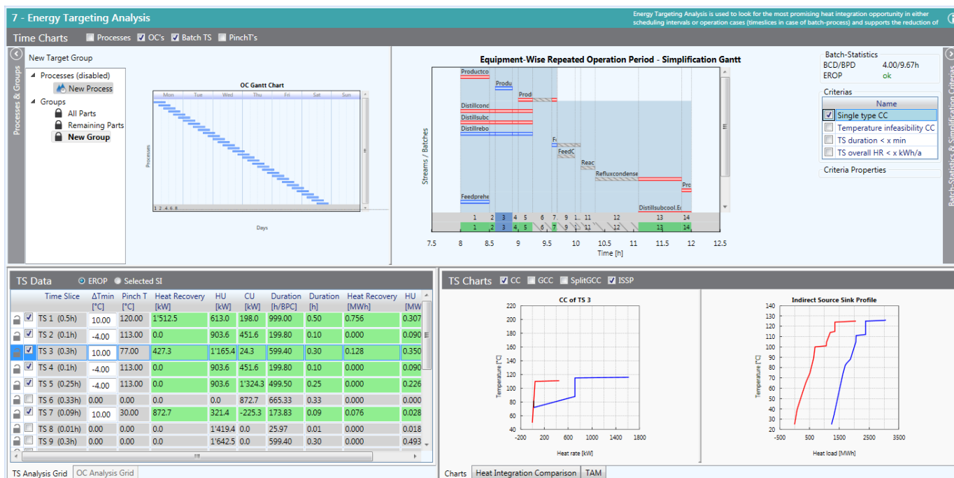
Figure 15: PinCH: screenshot of the Energy Target Analysis interface for simplifying repeated batch processes to most energy relevant time slices for direct heat recovery.
